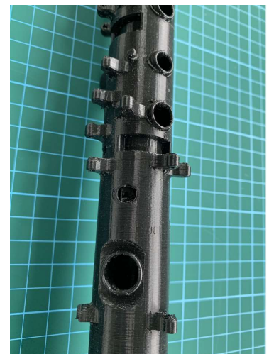
FDM printed clarinet joint by Sharon Jones.
