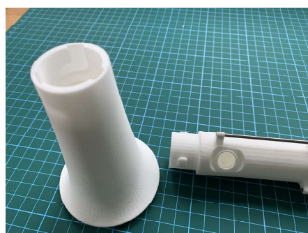
SLS printed components by Freddy Holdsworth, with pillars mounted by Peter Worrell.
