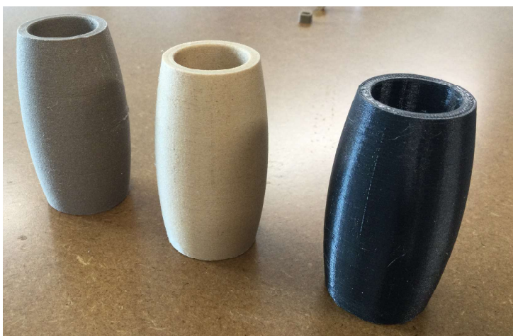
Barrel made from nylon, and two barrels made from wood fill by Sharon Jones.
