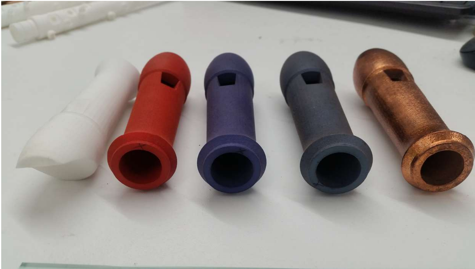
Experimental colouring of the white original 3D printed part (left) using coloured dyes and an electroformed copper coating (far right)
