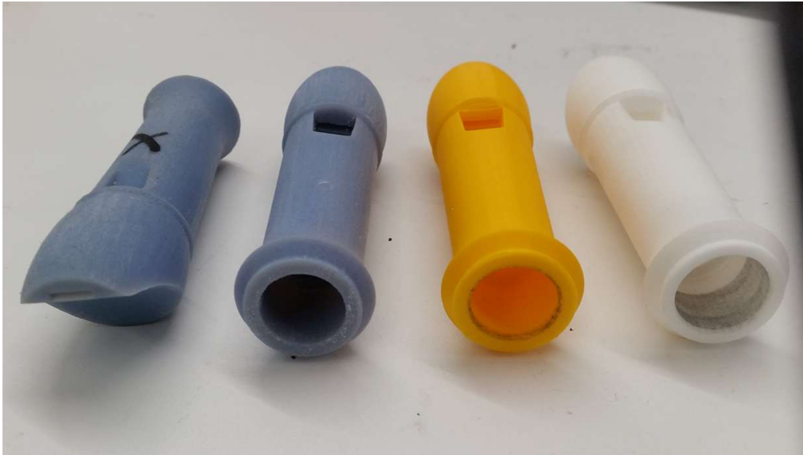
A selection of mouthpieces printed on different 3D printing technologies
