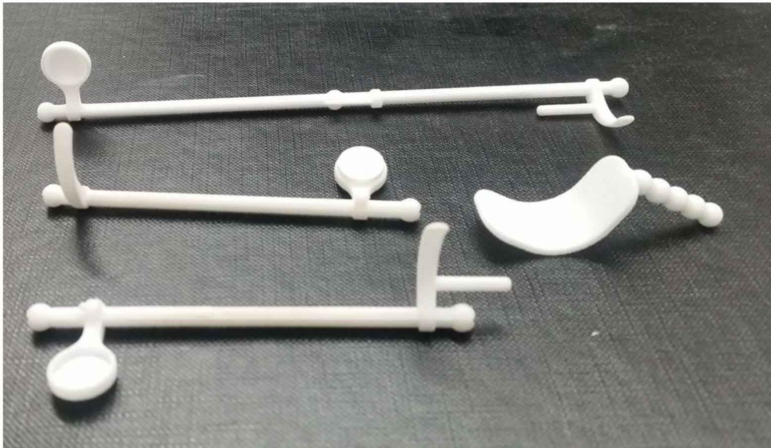
The rod assemblies printed in nylon
